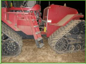
The victim was attempting to climb the tractor cab access ladder when he was run over by the moving left rear track.
