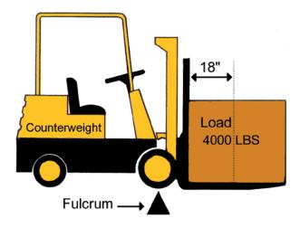
As the load is raised, it becomes possible for the forklift to fall to the side as well as tip forward. The operator must consider the center of gravity of the forklift and load together. This combined center of gravity moves as the load is moved and as the forklift travels over surfaces that are rough or inclined. Forklift Moment: 24" x 5,000 lbs. = 120,000 inch-pounds Load Moment: 18" x 4,000 lbs. = 72,000 inch-pounds
