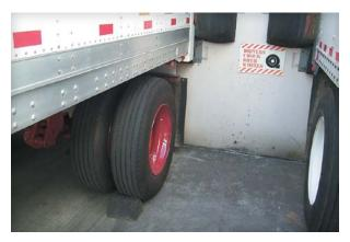
Trucks or trailers must be chocked or blocked at the wheels, or with a mechanical device that secures the truck or trailer to the loading dock. Notice the sign tells drivers to chock the wheels.
