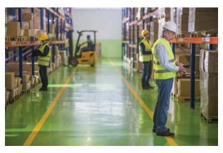
Mark aisles to help keep adequate clearance for forklifts.
