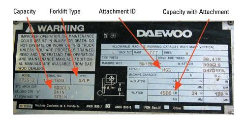
This LP Gas Forklift can safely lift 5,000 pounds 173 inches high with a center of gravity 24 inches from the face of the forks. With an attachment labeled "HSS," the safe load drops to 4,500 pounds.
