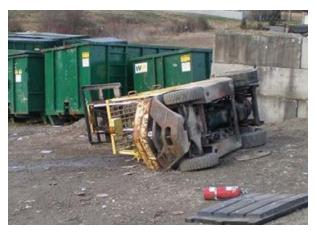
A forklift operator was pinned and killed when the forklift the worker was operating overturned.
