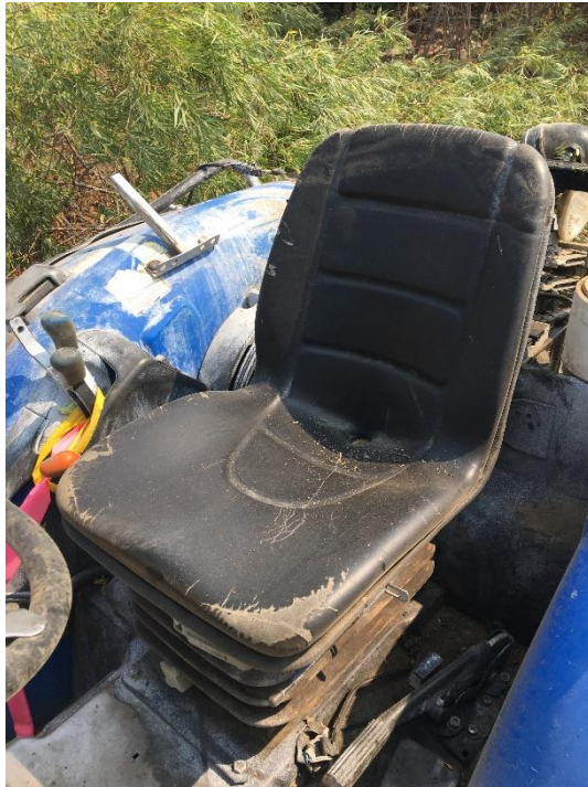
Photo 3. The tractor with its ROPS in the “down” position and no seatbelt installed.
