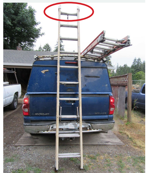
Figure 2: The fiberglass extension ladder involved in the incident was damaged. The top rung of the ladder was bent (circled). The damage was reported to the employer, but the ladder was not removed from service or fixed.
