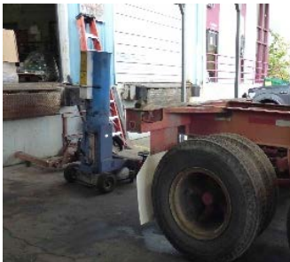
Work area where trailer crushed the mechanic against the blue steel bumper jack.
