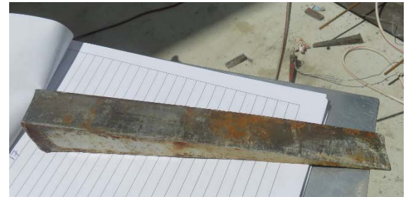
Steel wedge that was accidentally dropped 50 feet, striking an apprentice ironworker.
