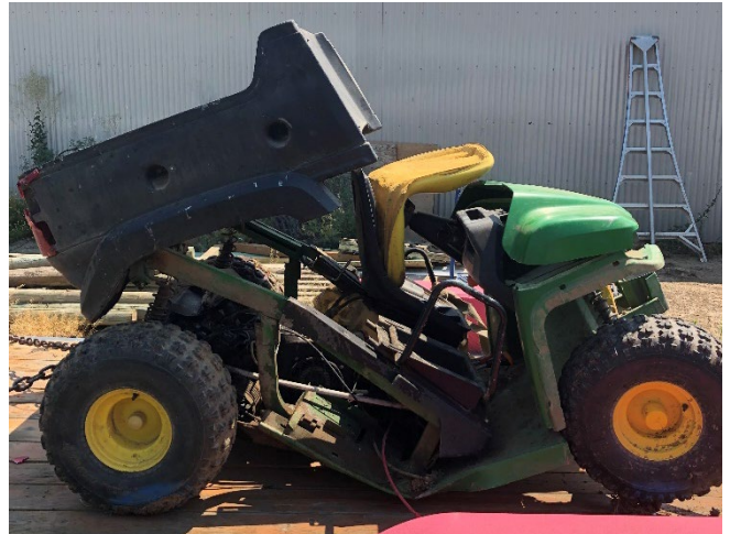
Utility Task Vehicle (UTV) with collision damage caused by passenger car.
