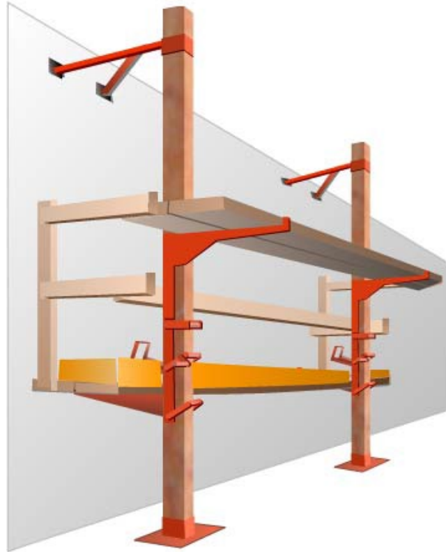
Illustration 1. Pump jack scaffold with workbench and guardrail. Courtesy of The Occupational Safety and Health Administration (OSHA).
