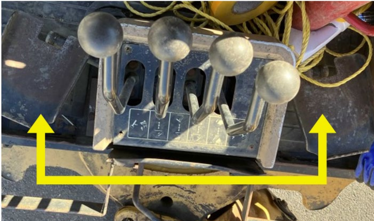
Photo 6. Foot pedals that control the backhoe boom swing.
