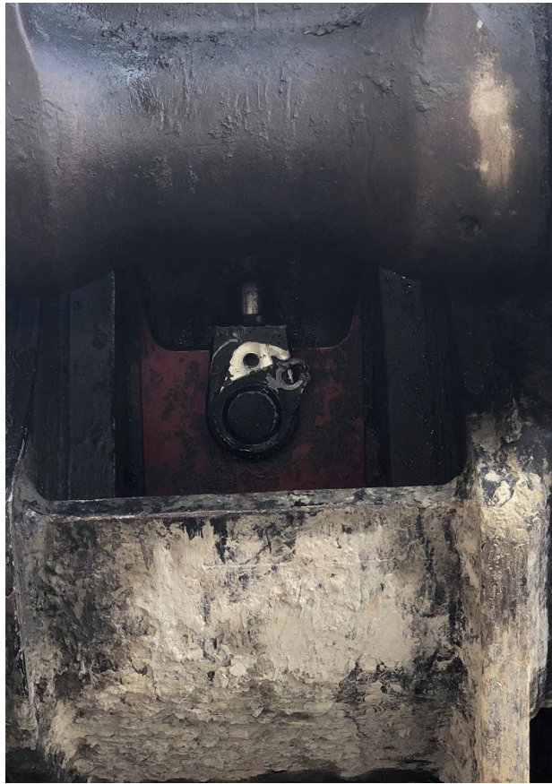
Photos 2 and 3. View of the wedge lock within the coupler on the left and close-up of the wedge in the unlocked position on the right.
