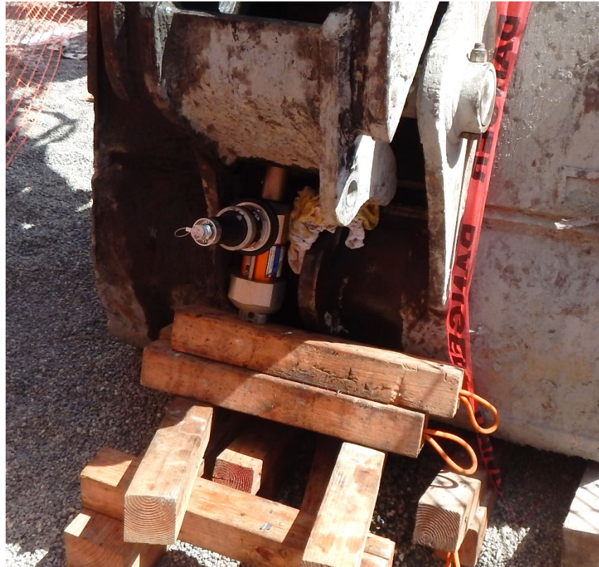
Photo 7. Bracing and tool that rescue workers used to stabilize the bucket and retract the wedge while trying to release the spotter's fingers.
