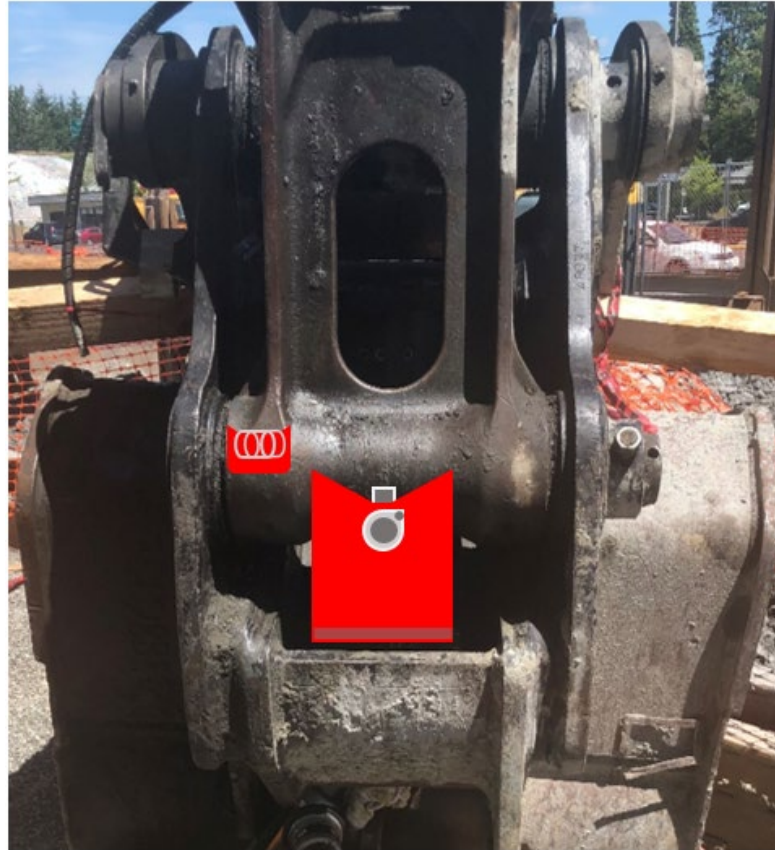
Photo 1. Quick coupler connecting bucket to excavator boom with illustrations of approximate locations of wedge (center) and safety knuckle (on left). Not to scale.
