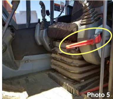
Photo 5 & 6. Example of intact hydraulic safety lock lever raised in "on" and lowered in "off" positions on a different machine.
