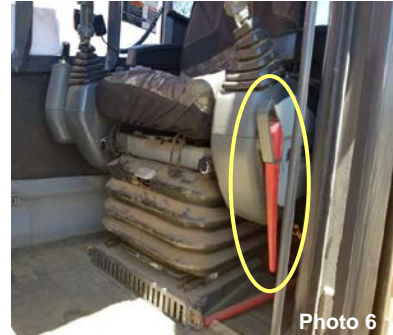
Photo 5 & 6. Example of intact hydraulic safety lock lever raised in "on" and lowered in "off" positions on a different machine.
