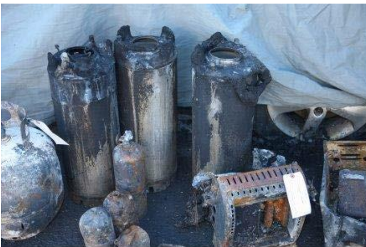
Photo 3: Incident propane cylinders and space heater.
