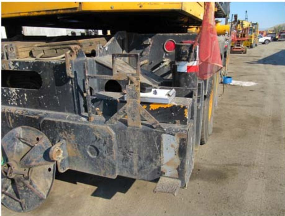
Photo 8. Incident crane rear access system where victim fell.
