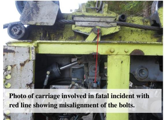
Photo of carriage involved in fatal incident with red line showing misalignment of the bolts.
