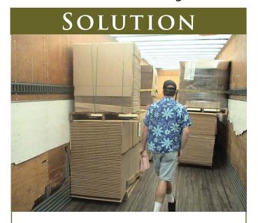
The top tier pallet is positioned so that the receiving customer's forklift driver can lift it.
