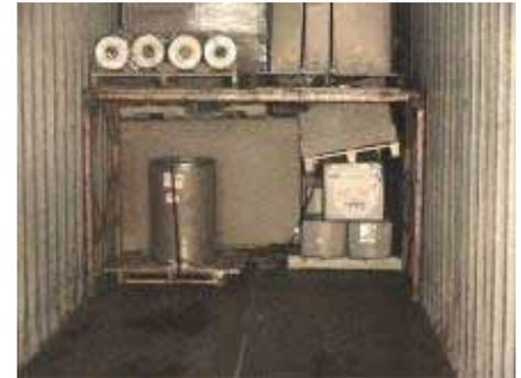
Secured freight supported by steel frame structure designed to accommodate two tier cargo stacking.
