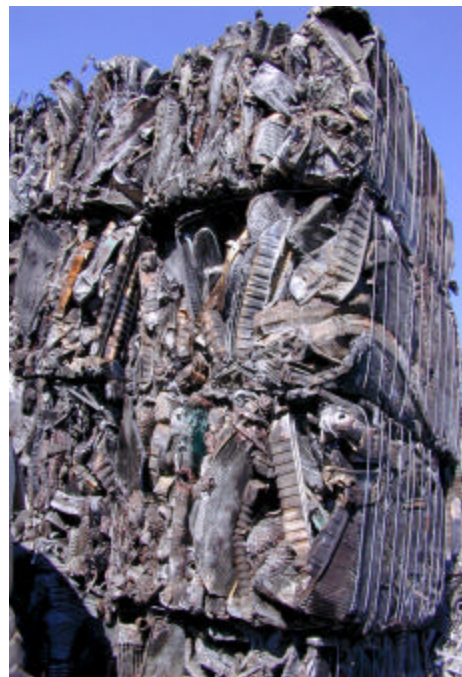
Disassembled car and truck radiators baled for shipping. Torching radiators to melt solder can cause severe lead poisoning in workers
