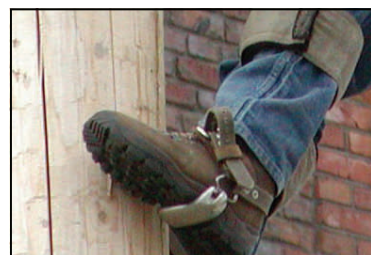
Hooks that are not securely planted into the pole can dislodge and cause a fall.
