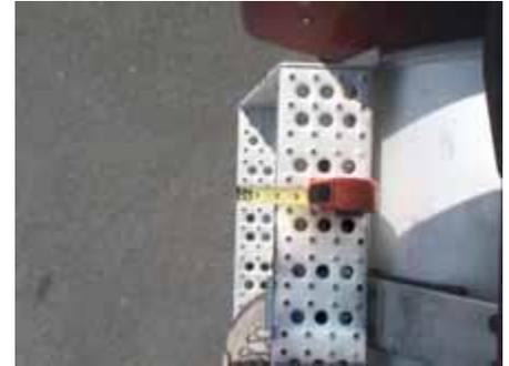
As shown here, the lower step is virtually under the top step. If the driver exits face forward there is minimal room for a foot to rest on the lower step and the foot is likely to slide off.
