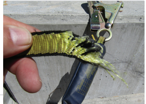
The exposed edges (shown above) cut a worker's nylon webbing lifeline (shown below) during a fatal fall.
