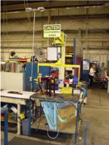
Hoist used to install stove faces, which can weigh up to 55 pounds.
