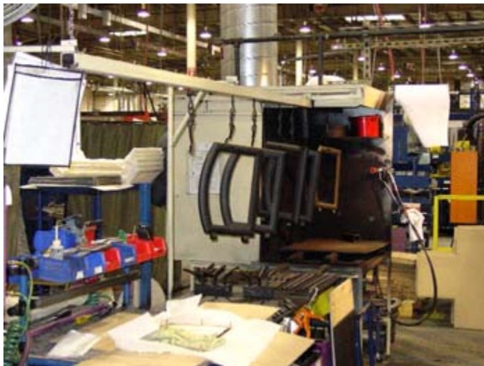
Recently painted stove doors drying on the hanger line. Doors will be assembled on the packaging material below.
