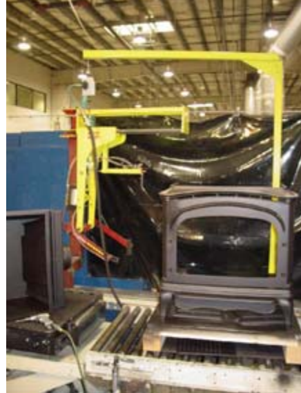
Hoist used to install engines in stove frames.
