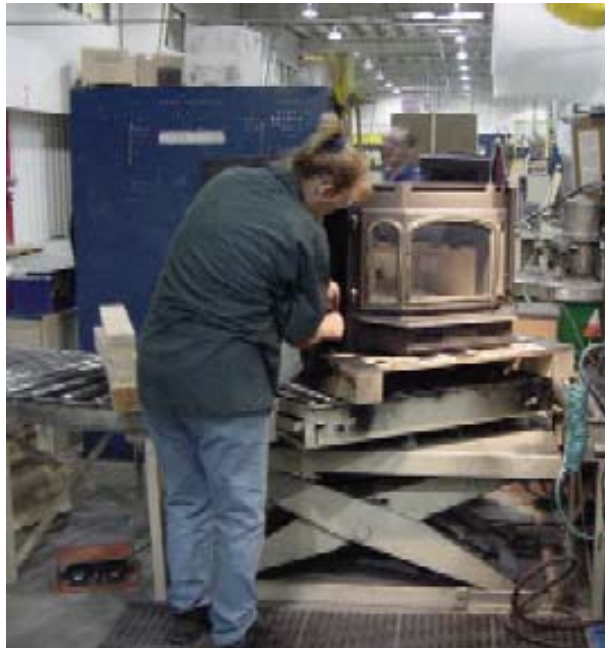
Scissor lift with turntable provides access to all sides of a stove during final assembly.
