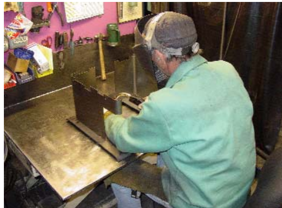
Welding workstations were specifically designed to allow seated work.
