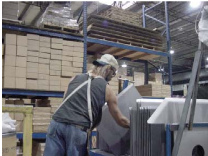
Lifting parts onto and off of carts can all be done between knee and waist level.
