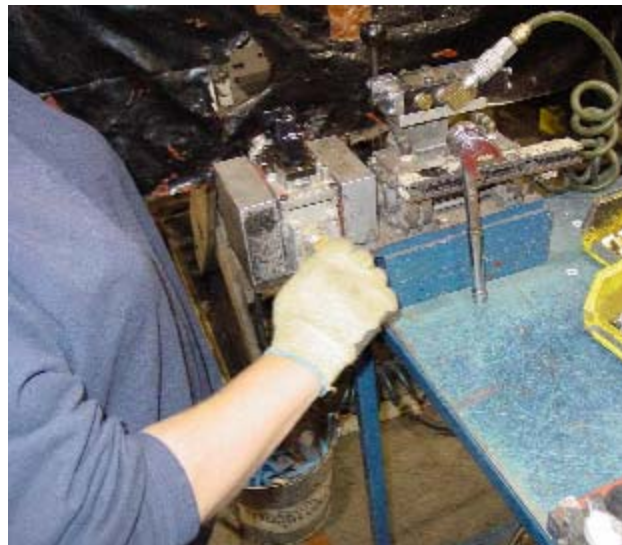
The clamp eliminates the need to grip the part and leaves both hands free to work.
