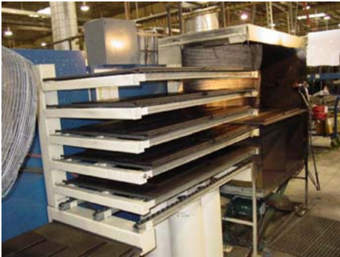
Parts storage on elevated shelving on the left, next to a height adjustable workstation on the right.
