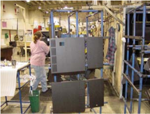
Custom-built mobile racks place parts at a good height and provide easy access to all sides.
