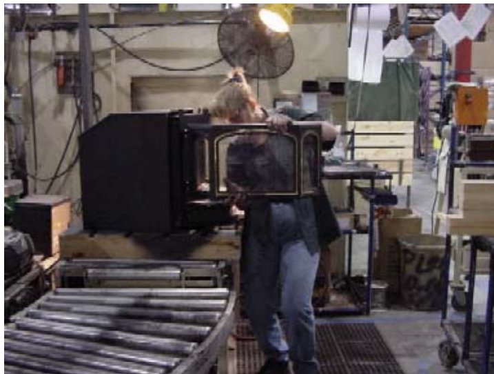
Workstations with rollers are built right into the line, so product flow is maintained.
