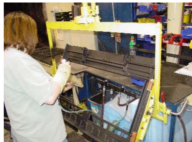
Hoists can also be used to position parts at a good height for some finishing tasks.
