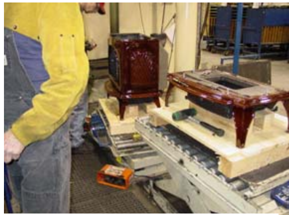
Adjustable workstations also allow a single employee to work with different size parts more easily.
