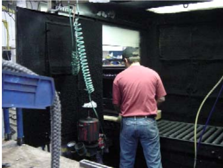
Using rollers to move a partially assembled stove from one process to another.
