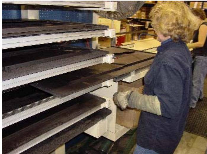
Adjusting the workstation to the same height as the shelf with the needed part allows the part to be slid across rather than lifted. Rollers on the shelving make sliding easier.
