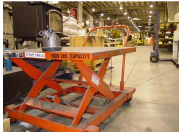
Larger, heavier parts can be moved and worked on using a mobile scissor lift.
