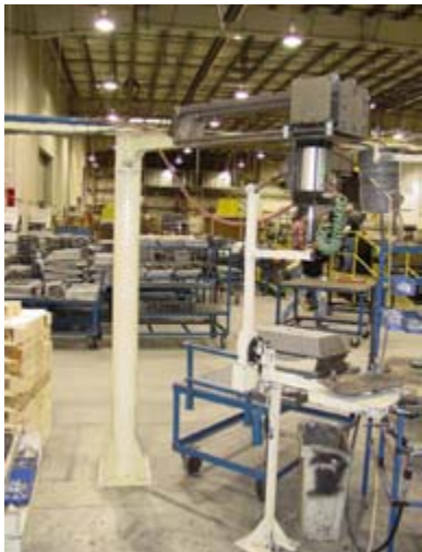
This hoist is specially designed to lift, move and rotate heavy cast stoves.
