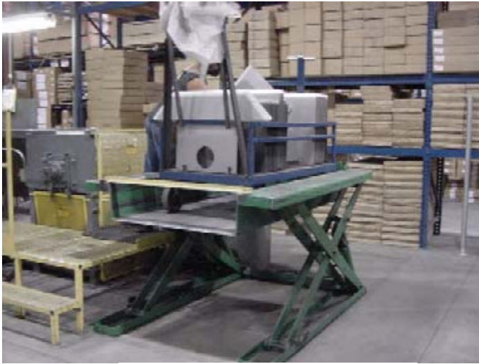
Cart on the lift table.
