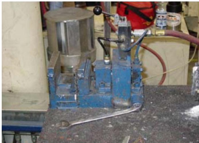
Pneumatic clamp used to hold valve parts during assembly.
