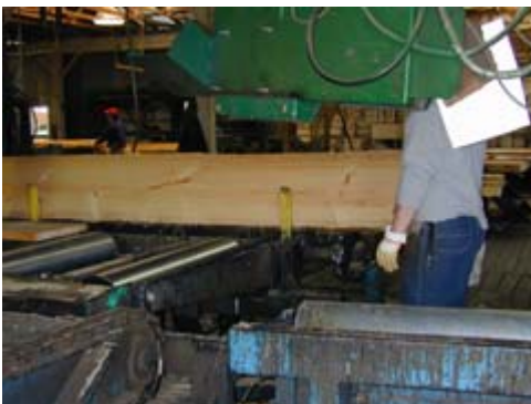
A "home-made" board turner assists the operator to turn the cants and so to eliminate the heavy lifting/turning activities at this job.
