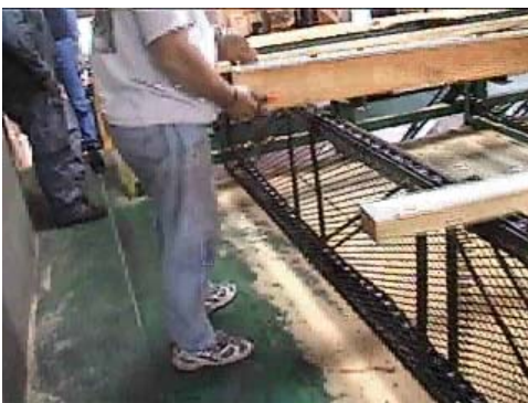
A grader is turning boards to inspect and grade them.
