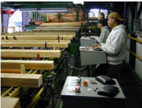
A board-turning system is installed at the grading stations, and graders do not need to manually turning and marking boards.
