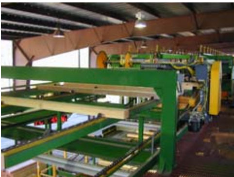
A mechanical sorting and stacking system is installed to replace the manual pulling and stacking process
