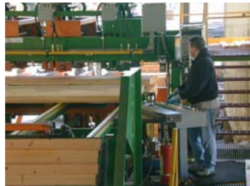
A mechanical sorting and stacking system is installed to replace the manual pulling and stacking process
