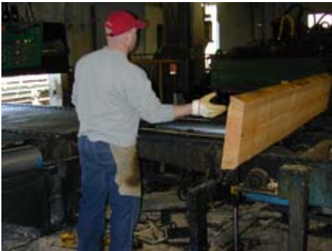
A “home-made” board turner is also installed at the edger station to assist turning cants.
