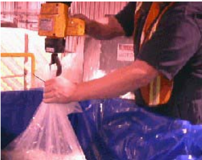
The new way: This hoist can lift multiple bags at one time.
