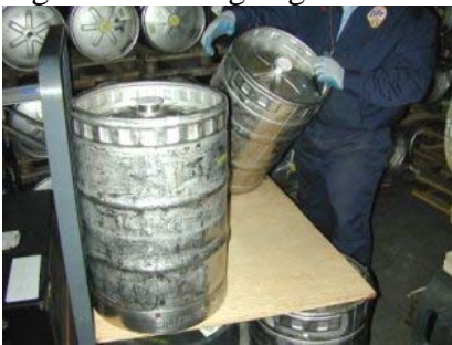
a) Improperly lifted from floor by only one worker (two workers required)
