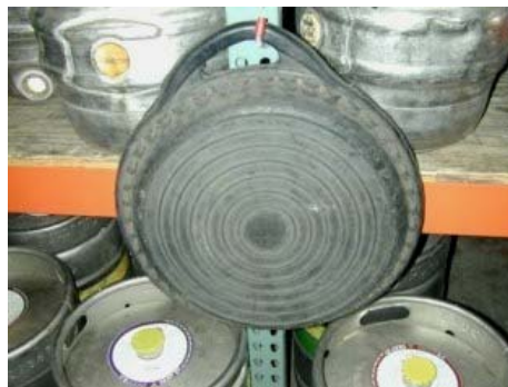
Figure 5. Rubber bumpers are used when dropping kegs from shelf level to floor level. (minimizes the need for heavy lifting (lowering) of kegs)
