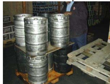
b) Edge rolled/slid from raised pallet on forklift (only one worker required)
