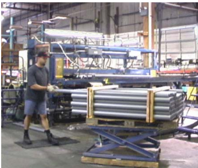
The new way: Using the scissor lift to raise the pallet so that pipe can be handled at a comfortable height
