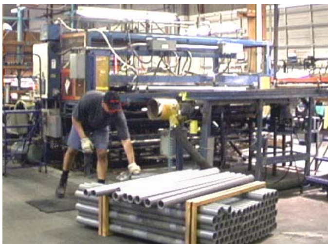
The old way: Bending over to pick up pipe from pallet on floor
