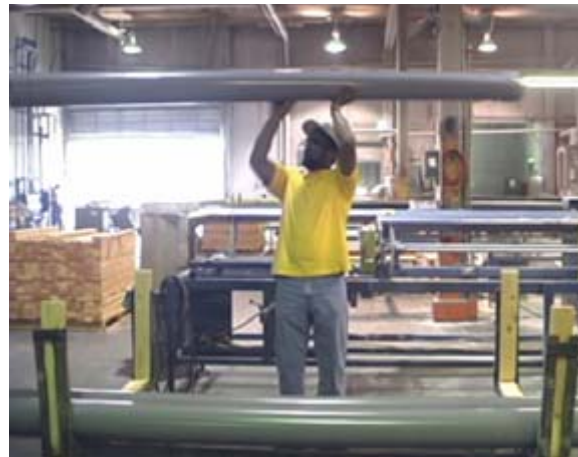
The old way: Lifting pipe overhead in order to rotate it
