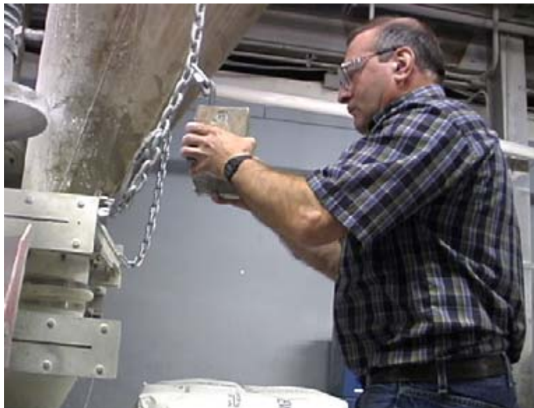
The new way: Hanging weights on hooks under the scale results in a less awkward lift
