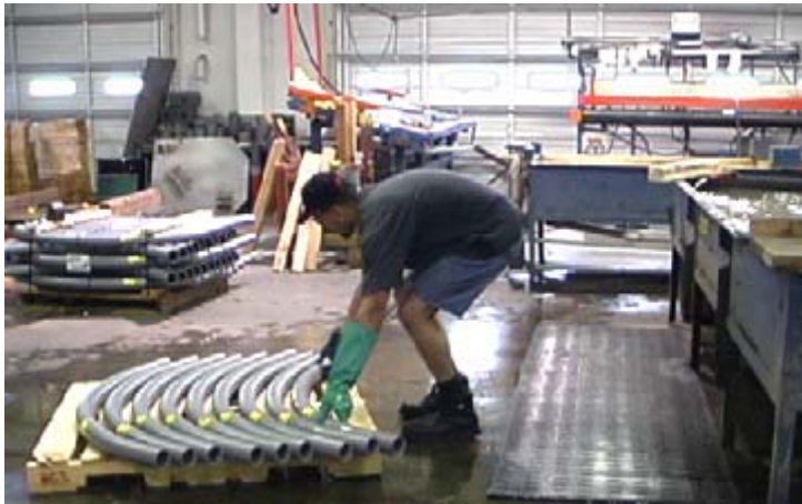
The old way: Bending over to place pipe on a pallet at floor level.
