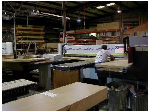
Figure 2. Panel saw workstation with scissor-lift for uncut wood shown on the left and transfer conveyor for finished wood shown in the foreground.
