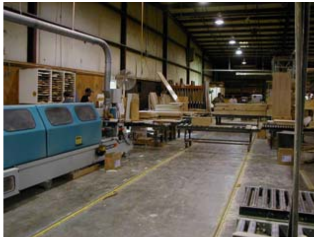
Figure 1. Roller conveyor system and roller transfer cart moving material in and out of the panel saw and the edge banding machines.
