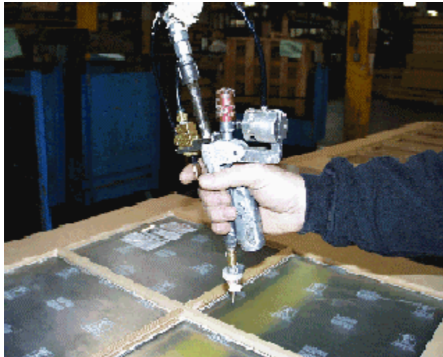
Figure 2: home made glue applicator (air pressure)
