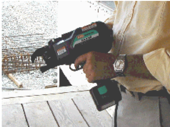
Figure 2. A rebar tying tool used by Utility Vault to secure reinforcement.
