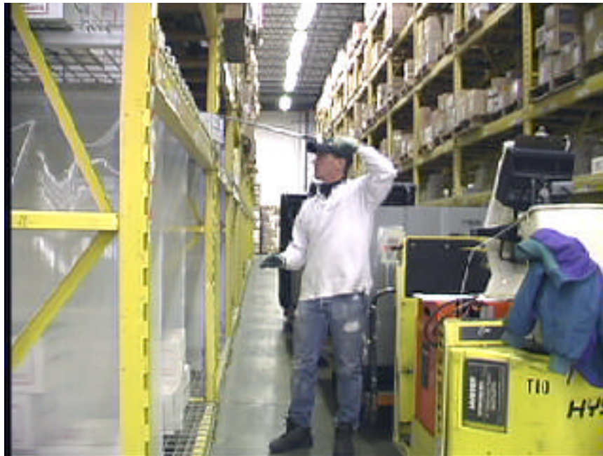
An Order Filler demonstrates use of a simple hook to pull items to the front of the bin for better lifting technique.
