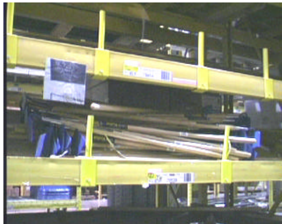
Storage bins are constructed with a floor slanting forward easing access for both Stockers and Order Fillers.
