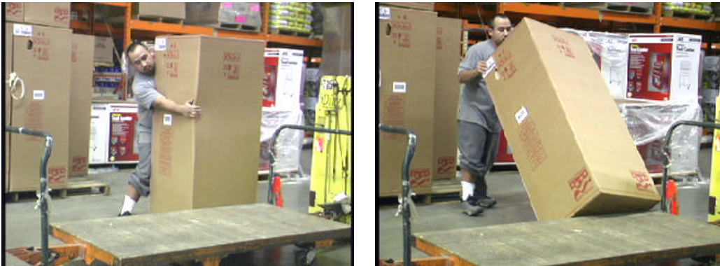
Left photo: New employees may try to "bear hug" lift a waterheater onto their cart. Right photo: Targeted employee training creates hands -on learning opportunities to practice correct material handling methods, such as using leverage to slide a water heater into position.
