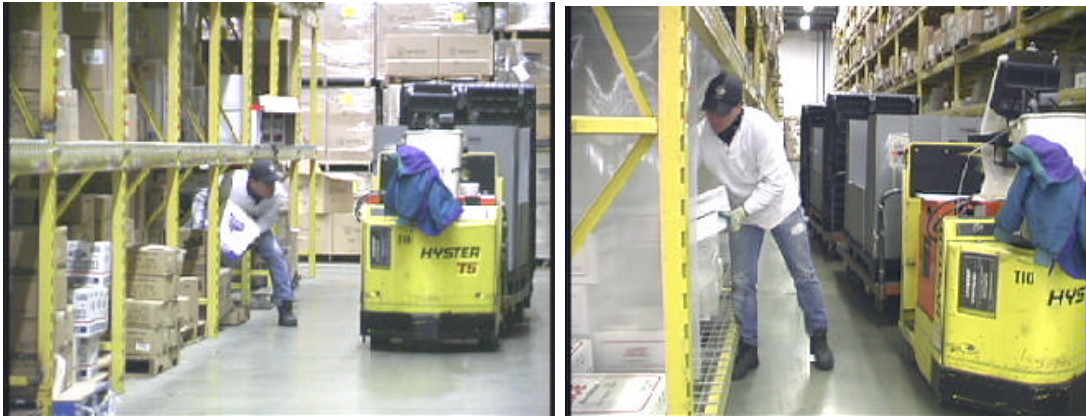
Left photo: Lifting conditions before improved controls were implemented. Right photo: Full Case Orderfiller demonstrates improved lifting posture due to warehouse reprofiling project that raised both the height of storage bin from the floor and increased maximum headroom.
