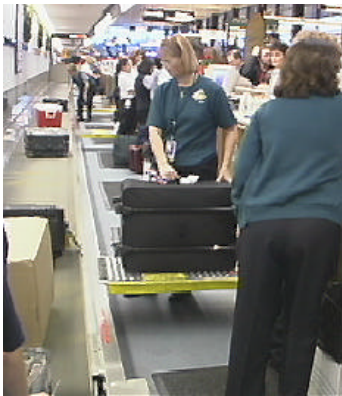
Rollers provide a place to rest bags until an opening appears on the conveyor
