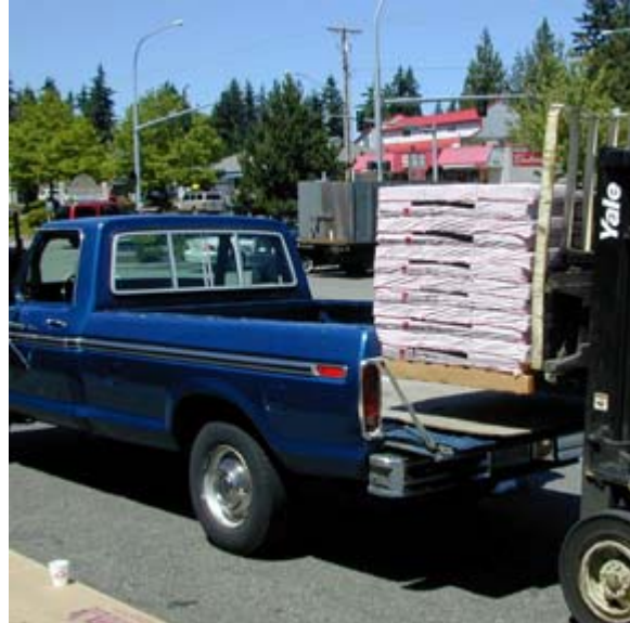
b) Loading a pallet with a forklift
