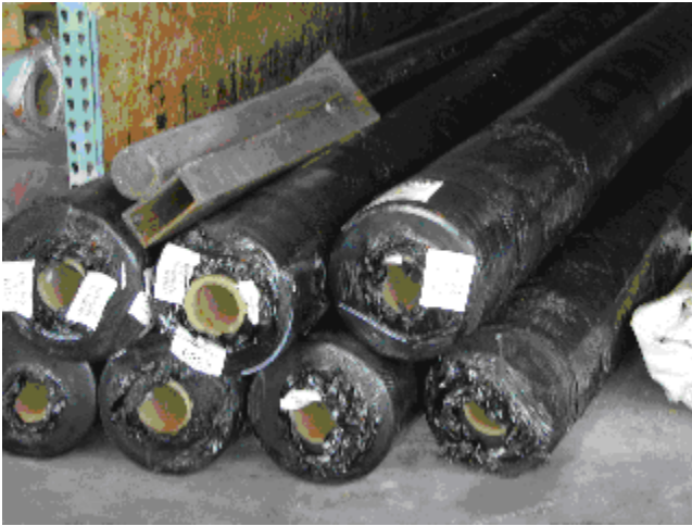
Figure 2. Forklift tong for rolls (on top of pile).
