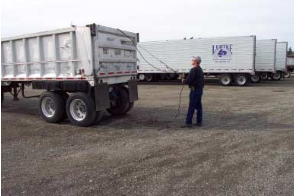
Employee uses an electric tarp device to deploy the tarp across the top of the container while pulling on the tie-down ropes.
