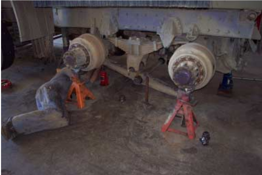
Employee using hydraulic jack to lift one end of the walking beam before securing it to the truck underbody. This is an alternative to two employees manually lifting the assembly.
