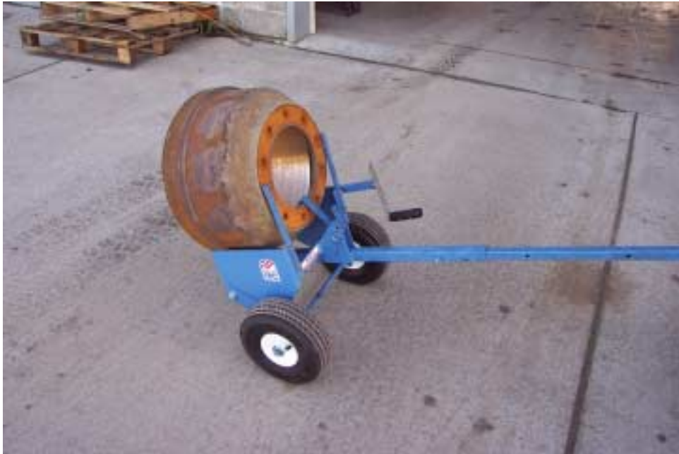
Drum dolly with hand crank can lower or raise the drum dolly to the proper level.
