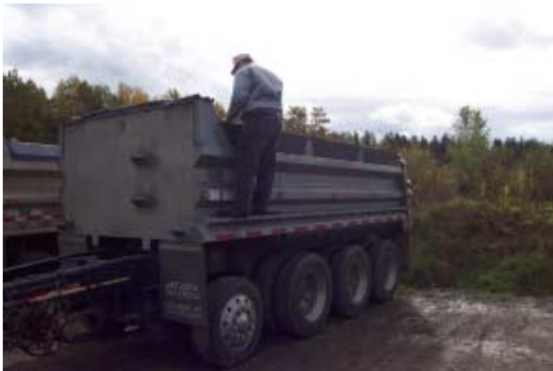
Employee stands on running toe rail installed on side of truck to reduce the risk of slip and fall injuries.
