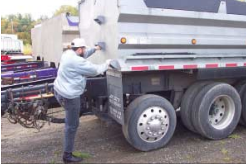
Worker uses handholds that were installed to reduce the risk of injuries from falls.
