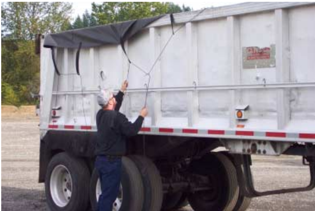
Employee hooking down the sides of the automatically deployed tarp.
