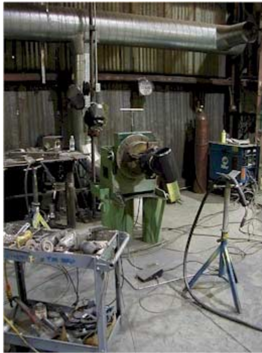
Figure 3. Rotating-welding jig to hold parts and place work area in position.
