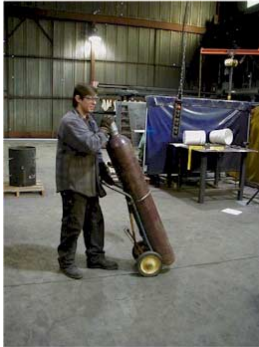
Figure 9. Use of a handcart to move gas cylinders.
