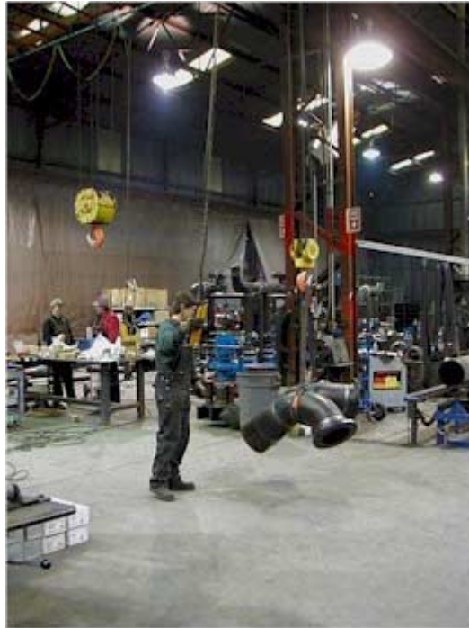
Figure 7. Lifting a pipe piece with an overhead crane.
