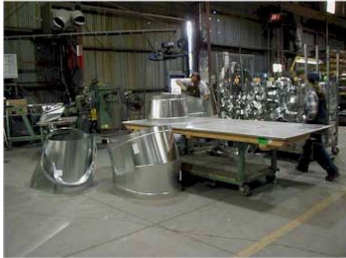
Figure 5. Use of a cart for storage and working on sheet metal ductwork.
