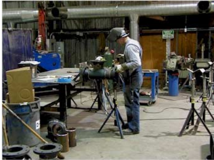
Figure 2. Welding with a holding jig and stand.
