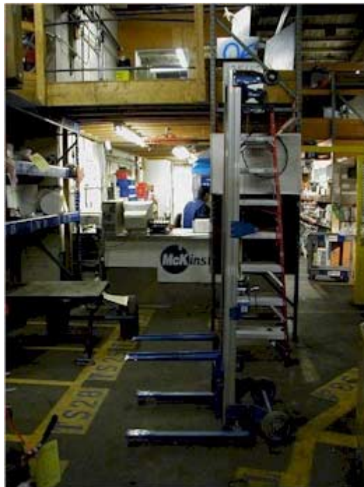
Figure 8. A lift used in the tool room for placing/retrieving material over the head.
