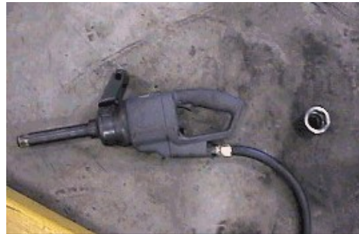
New impact wrench does the same job at less than half the weight
