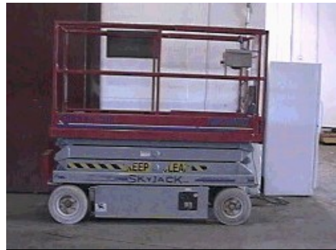
The powered man-lift is used daily to work high on equipment, change light bulbs, clean and paint high walls, etc.
