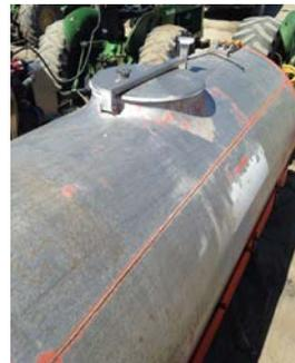
**Warning: Confined Space!** Stop and do not put any part of your body through the opening of a confined space like this metal tank if your employer doesn't have a required written confined space entry program that includes the tasks you perform.
