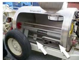
Airblast sprayer tanks and other confined spaces might have dangerous moving mechanical parts inside (see arrows in photo to left). Accidental start-up or release of built-up or stored energy during maintenance pose serious injury risks to workers.
