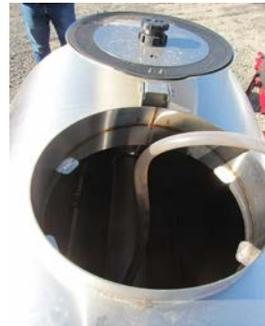
**What you don't know can harm you.** Entering an airblast sprayer tank like this one or other confined space to inspect, clean, maintain, or make repairs requires that your employer provide you with special safety training, equipment, and written procedures..
