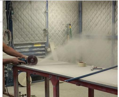
Grinders not equipped with a water delivery or vacuum dust collection system put out a lot of harmful silica dust, as shown above.
