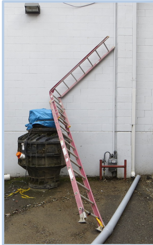
Incident scene with broken 24-foot fiberglass ladder.
