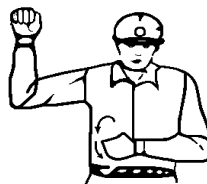
FOR MOBILE CRANES LOCK THE CRAWLER BELT ON SIDE INDICATED BY RAISED FIST TRAVEL OTHER CRAWLER BELT IN DIRECTION INDICATED BY REVOLVING FIST
