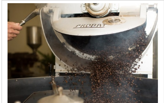
Air testing results show that substantial amounts of potentially harmful diacetyl and 2,3-pentanedione vapor are released when unflavored coffee beans are processed.
