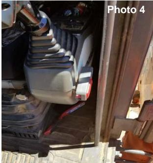
**Photo 4.** Broken hydraulic safety lock lever on processor.
