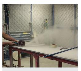
Grinders not equipped with a water delivery or vacuum dust collection system put out a lot of harmful silica dust, as shown above.
