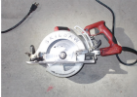
The framer was using the saw to make a cut when it kicked back, cutting through his boot.
