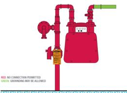
Bonding on the wrong side of the meter does not bond the interior piping and can lead to a gas leak, injury or a structure fire. Avoid return trips, always bond on the customer side of a natural gas meter!
