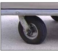
This was the second caster tried. The tires would sink and grab at the ground or floor covering. This resulted in push and pull forces that exceeded recommended limits.
