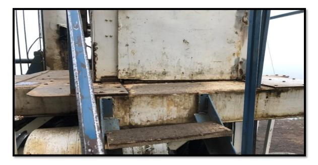
The deck surface of the yarder is worn down to bare metal and is needing repaired.
