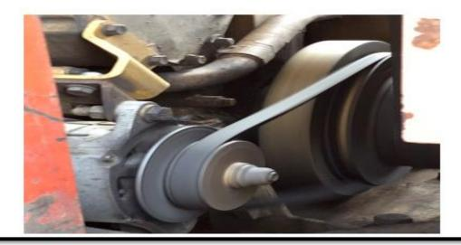
In accordance to WAC 296-54-573(40) Each machine must be equipped with guarding to protect employees from exposed moving elements, such as, but not limited to, shafts, belts, pulleys on
