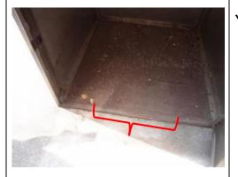
The plywood lip created a barrier for the central wheel of the spring-loaded bin; the wheel wore out the plywood.
