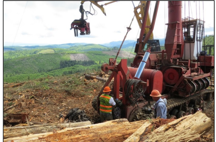
Incident landing site with yarder and processor.
