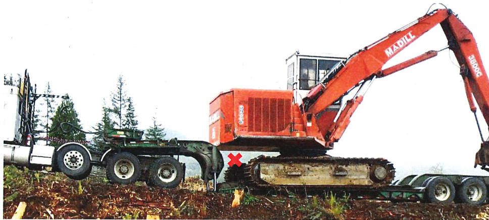
Incident scene showing the position of the operator (X) when the trailer detached from the gooseneck.
