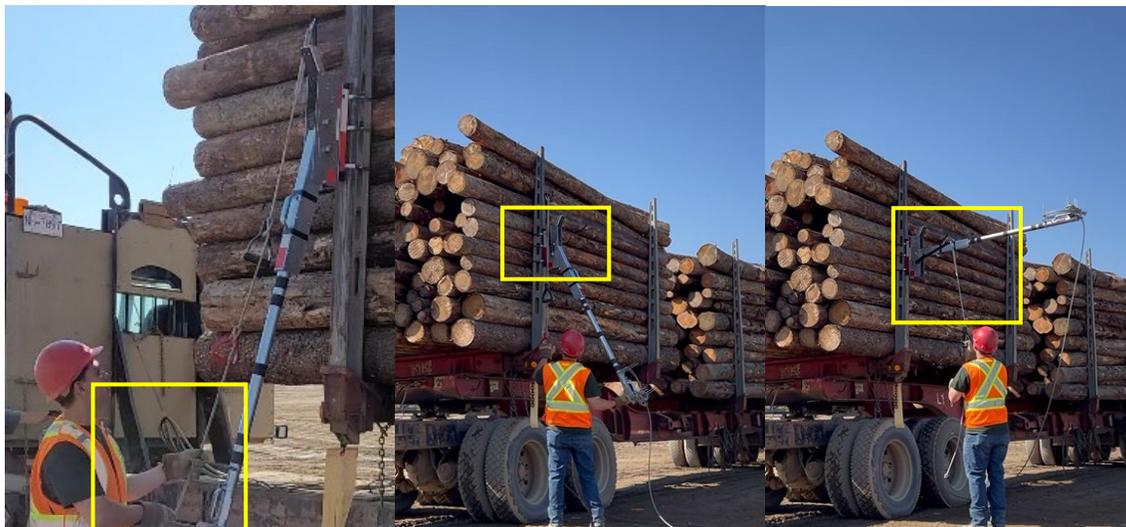
Figure 30. Use of sling rope for preparing for slingshot motion.
