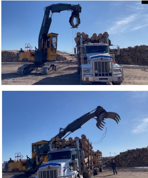
Figure 8. Loader draping the wrappers over the load.
