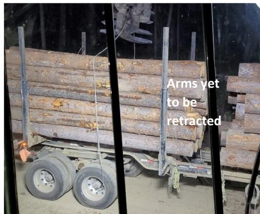
Figure 15. ExTe Long Life arms yet to be retracted to the rested position.
