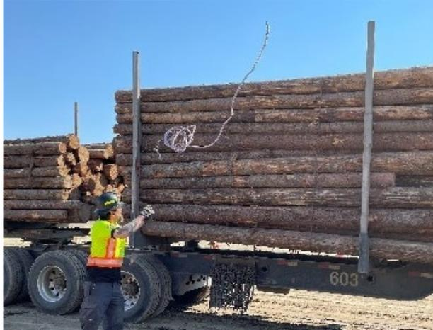
Figure 32. Driver throwing a synthetic wrapper.
