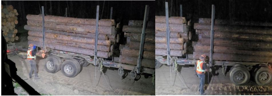
Figure 13. Driver setting up wrappers on the loader-assist tools at nighttime.
