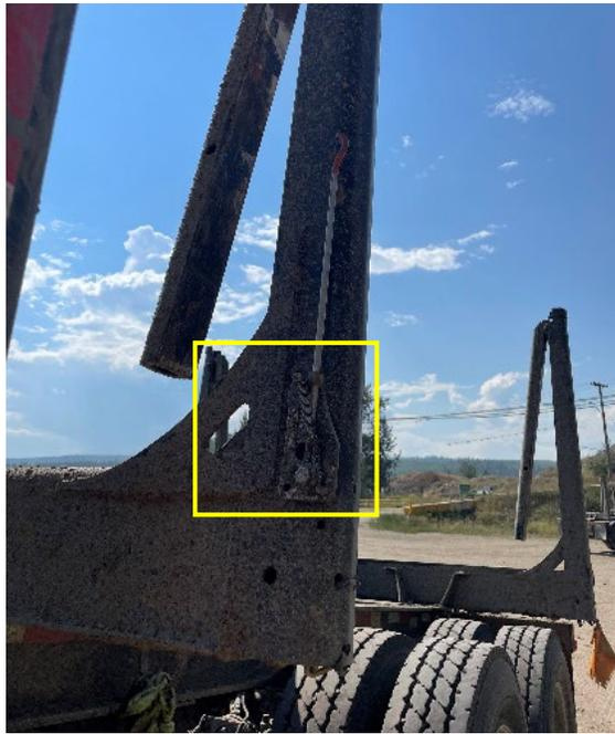
Figure 18. ANR SLM installed 2 ft lower than optimal on the stake creating the possibility of grapple hitting the tires.
