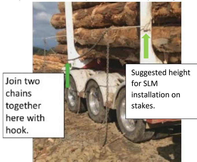
Figure 19. Chain arrangement on the arms of the spring load mechanism used in Australia (image source-ANC Forestry, reproduced with permission).
