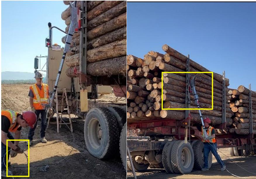
Figure 29. Placement of the other end of wrapper before the slingshot motion.
