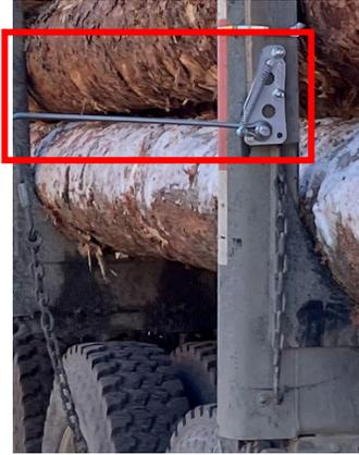
a) ANC spring-loaded mechanism (SLM)
