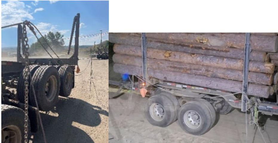
Figure 6. Arrangement of wrappers on the arms of the spring-loaded mechanism.
