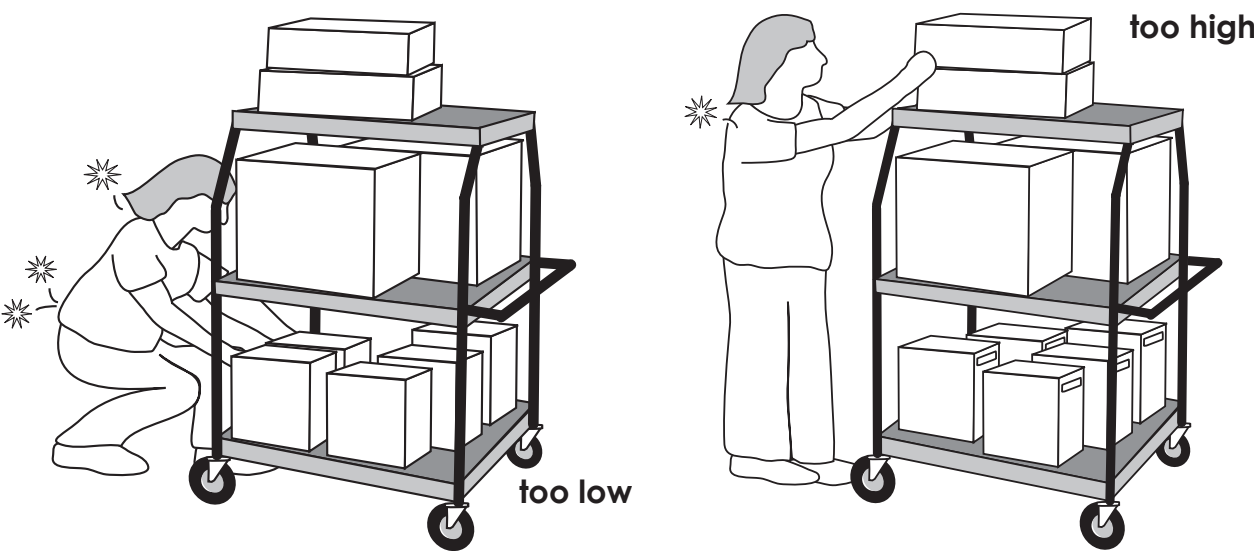
Figure 4.9 High shelves can lead to awkward shoulder postures. Low shelves can lead to awkward neck and back postures.
